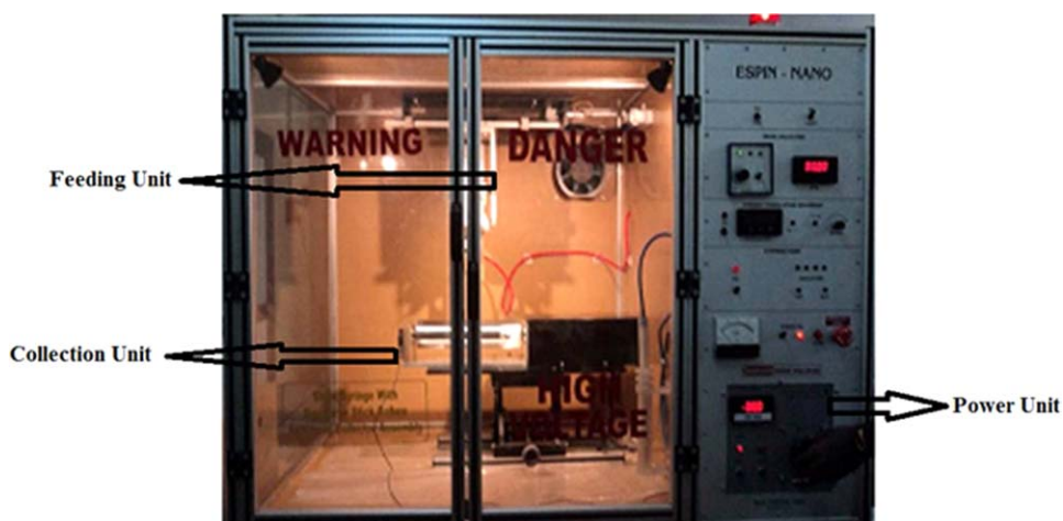
Figure 1. Photographic diagram of the electrospinning method. [Color figure can be viewed in the online issue, which is available at wileyonlinelibrary.com .]
